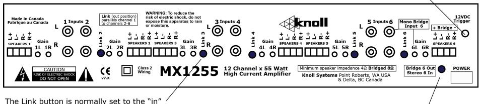
The Link button is normally set to the "in" position to give all six stereo inputs individual sources. When the Link button is set to the "out" position, that input Left/Right is linked or cascaded (or paralleled) to input #1 (without the use of Y cords). Any or all combination of linked inputs 2 to inputs 6 are possible. When all inputs are linked to input 1 the input impedance is about 4000  $\Omega$ .
